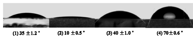
Figure 1. Static contact angles ( \theta ) to water for various glass plate surfaces, where the meanings of (1), (2), (3), and (4) are the same with those explained in Scheme 1.
